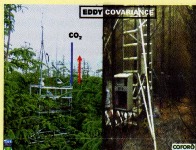
Figure 3: Real-time measurements of CO 2 exchange between the atmosphere and a forest ecosystem using eddy covariance equipment located above and below the forest canopy.
